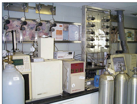
Sulfur Compound Gas Mixtures: Automated GC Analysis System
